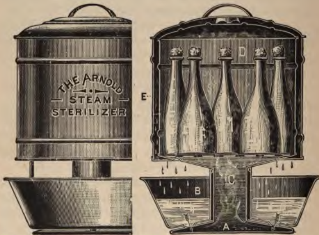
The Arnold steam sterilizer for sterilizing milk.* A, shallow copper steam generator; B, reservoir or pan; C, steam funnel; D, sterilizing chamber; E, hood.
